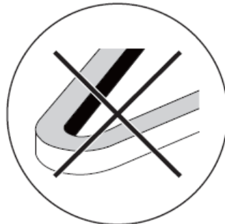
Bend too tight
