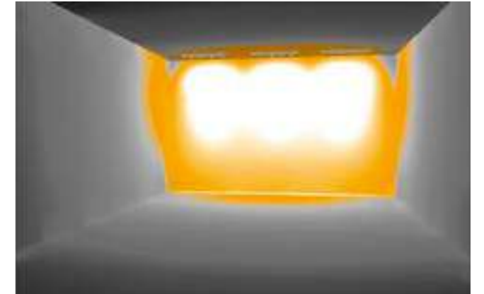
Luminaires at 600 mm offset from wall
