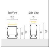
VarioClip SV 30mm (301/1.4310/V2a) Mounting clip for
