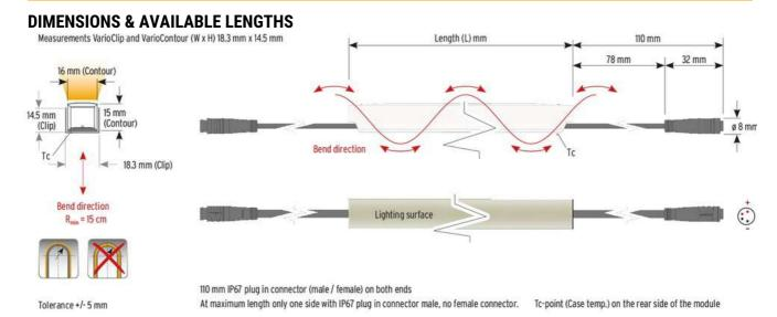
Fixture build to length (not field cutable): L = (N x 62.5 mm) + 26 mm; N = 3 ... 80; L min = 213.5 mm: Nmax = 80; L max = 5,026 mm
