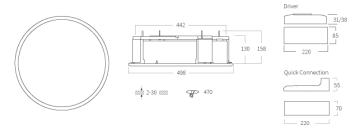
A recessed luminaire in a Robust IK 10 design. High level of efficiency and light comfort. Bevelled outer edge that provides a soft luminance transition to the ceiling. Front ring fastened with a safety screw to prevent access and disassembly.
