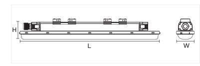
Material: White injection mould PC base Diffuser: PC Body Color: () Optic: 90° Power: 18W /36W / 50W CCT: 4000K Mounting Type: Ceiling Surface Ingress Protection Rating: IP65 Impact Protection Rating: IK10
