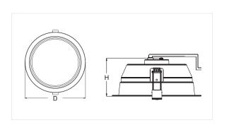
Material: Die-cast aluminium. embossed aluminum reflector. Diffuser: Opal Body Color: () Optic: 90° Power: 10W / 15W / 20W / 30W Ingress Protection Rating: IP44/IP20 Impact Protection Rating: IK08 CCT: Adj. CCT 3000K / 3500K / 4000K Mounting Type: Reccesed.
