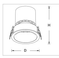
Material: Die-cast aluminum. Embossed aluminum reflector.
