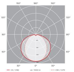
771-Orient +50°C, 5ft (2x1500mm)\*, Philips Fortimo LED Strip HV6, 70W, 9900lm, PC
