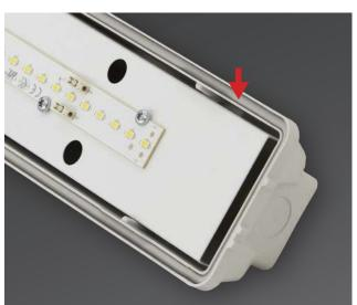
In order to ensure maximum heat, chemical and weather  $\textbf{resistance} \ \text{even under tough conditions, the } \textbf{gasket} \ \text{between}$ the diffuser and housing is made of silicone foam with enhanced resistance.
